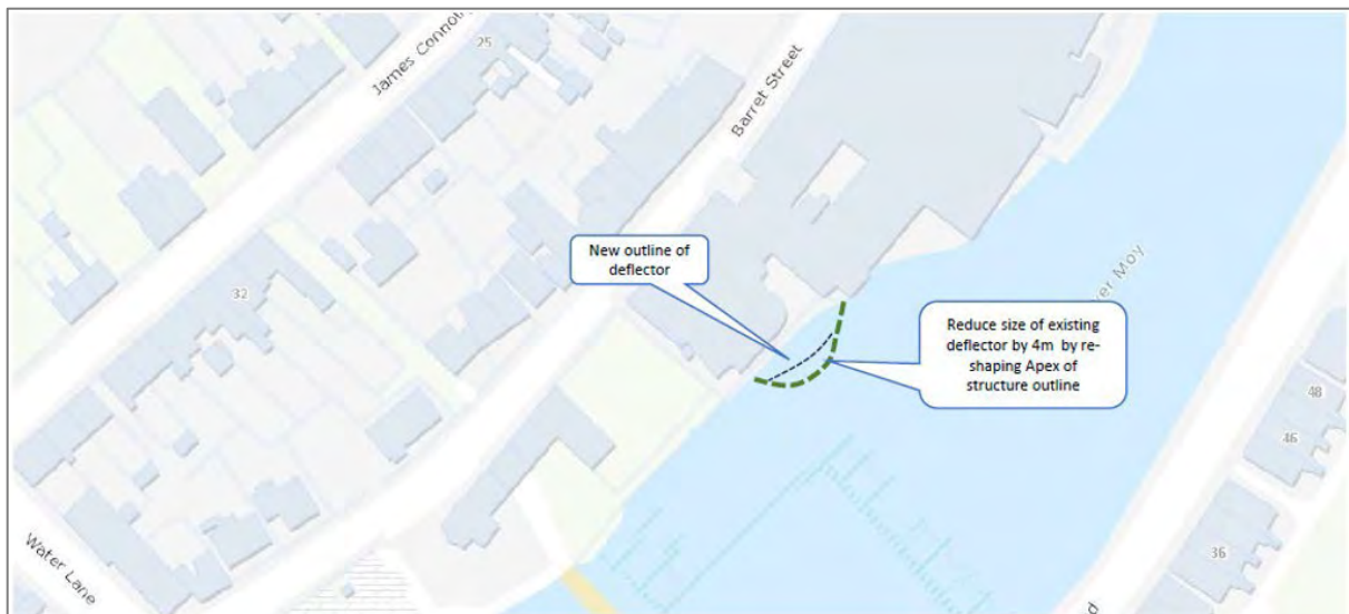
Figure 5: Proposed instream enhancement of Ridge Pool, showing reshaping of 'groyne' (Courtesy of RPS).
